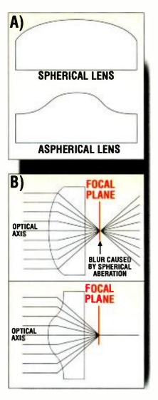
Figure 3. Light passing through the outer area of a lens focuses at a different point than light passing through its center. Fujinon uses an aspheric-shaped lens to correct for the distortion.
