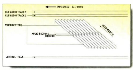
Figure 4. Recording track layout used for Digital-S.
