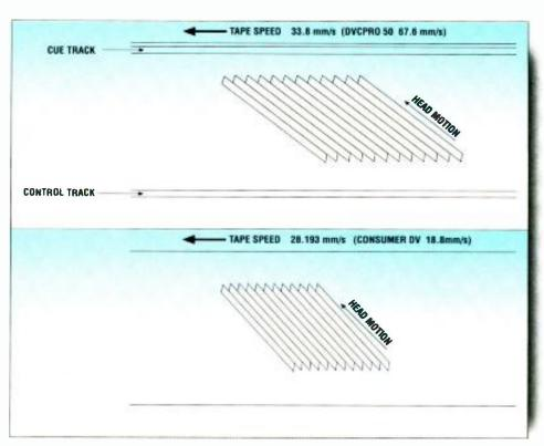
Figure 5. Track layouts for 6.35mm DV-recordings. DVCPRO (top) uses an 18-micron track pitch. DVCAM (bottom) uses a 15-micron track pitch, with the consumer DV format using a 10-micron track pitch in the standard mode. All three formats record audio, video and subcode information digitally on the helical scan tracks.
