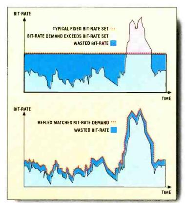
With fixed-bitrate encoding, either wasted space occurs or peaks exceed channel allocation. NDS Reflex matches the needed bitrate-to-channel-space allocation.
