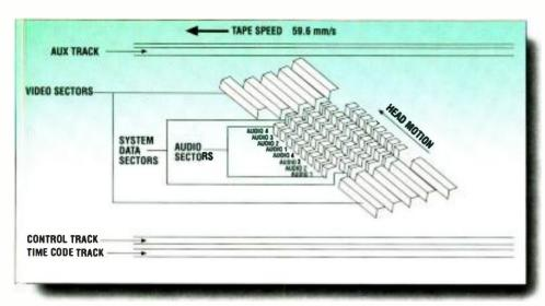
Figure 3. Tape layout used for Betacam SX.
