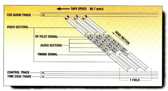
Figure 2. Digital Betacam's track footprint.
