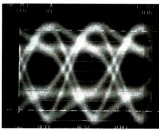
Figure 3. Signal shown in Figure 2 after high-frequency loss equalization. After reclocking, the signal can now be properly decided.
