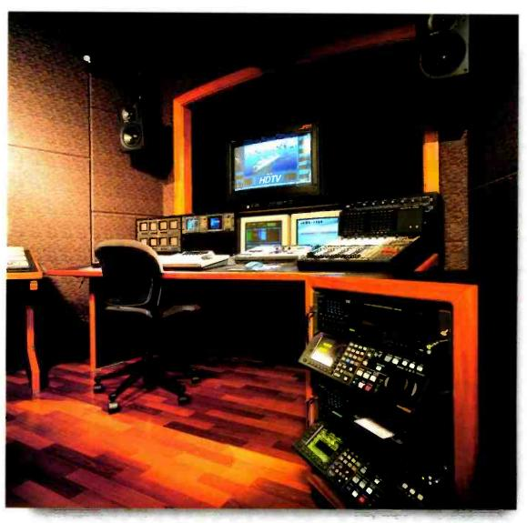
American Production Services' HD edit suite includes a Sony three M/E HDS-7000 production switcher, a two-channel HDME-7000 for creating 2-D and 3-D effects and Sony HDCAM HDW-500 VTRs in foreground.
